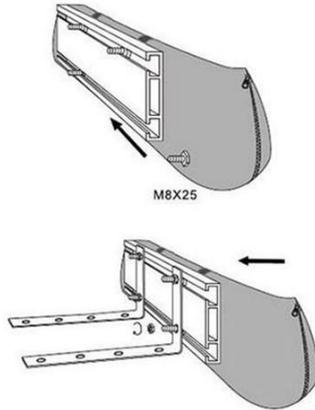
Install the awning to the L bracket using M8x25 bolts.
