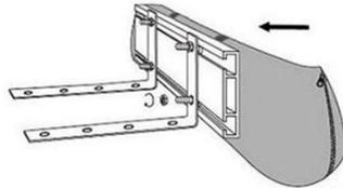
Install the awning to the L bracket using M8x25 bolts.
