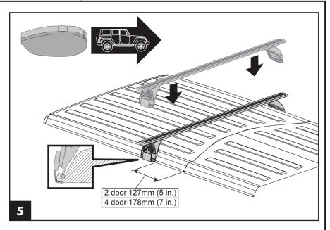
6) Remove the protective tape from crossbar. Place one crossbar in the rear position. Orient the thick side of the crossbar toward the front of the vehicle.
