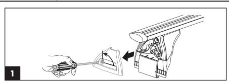
2) Loosen clip bolts using 4mm Allen wrench. Do not remove.
