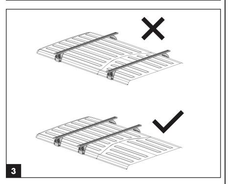
4) If necessary, tower spacing can be adjusted. Use the 4mm Allen wrench to loosen tower screw 1-2 turns. Adjust spacing, and re-tighten to 3.5 Nm.
