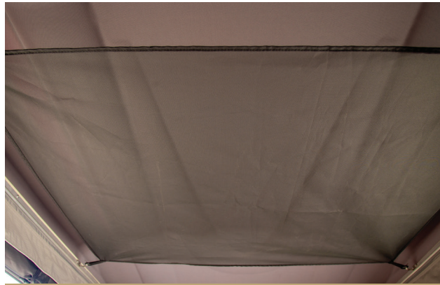
Roof Mesh Light Storage
